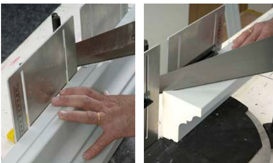
WINDOW SILL PROFILE ANGLED ON BOTH SIDES
